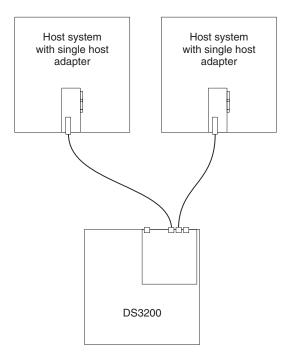
Figure 28. Single-controller direct-attached connection to single HBAs in multiple hosts
